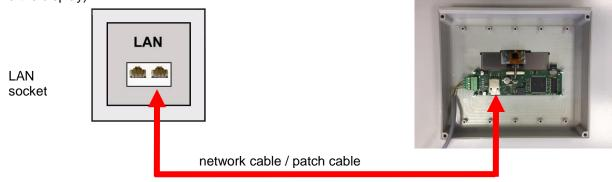
Wait until you have connected the osf control unit to an active network socket before switching on the power supply. The osf web server in the osf control unit then automatically locates the osf communication servers and registers itself with the server databases.
