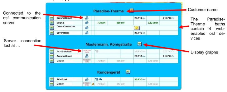
In order to use the communication server, the option "Use communication server" must be enabled in the control unit itself (default factory setting):
